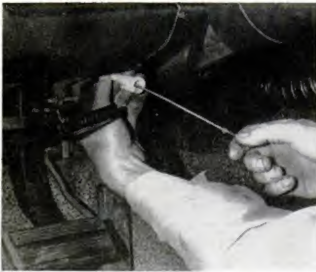
IN TRANSMISSION PINION SYSTEM, detach cable from speedometer head, then pull it from housing
